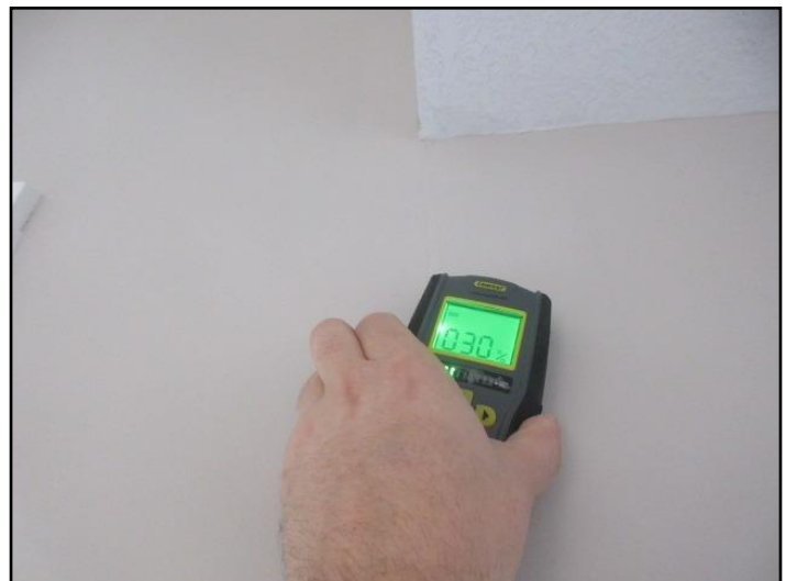
High Moisture Found On Exterior Rear Wall MB
